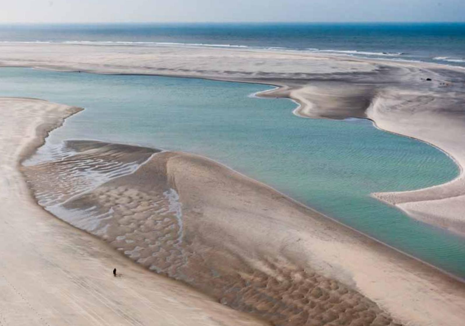
In 2011, the coastline to the south of The Hague acquired a hook-shaped peninsula made of sand: the Sand Motor. Wind, waves and currents are spreading the sand from the Sand Motor gradually along the coast in both directions, preserving the coastline, and creating new nature and a dynamic recreational area. This is Building with Nature. Since the Sand Motor was established, there has been extensive research into how this innovation is working.
